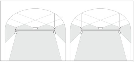
A square suspended light structure with uplights for indirect lighting is installed in each vault. Spotlights can be mounted on the lower part of the structure for accent lighting.
